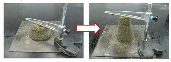
Before adding TG Rock-W Mini slump value: 8 cm Texture: Has fluidity After adding TG Rock-W 1.0 kg/m<sup>3</sup> Mini slump value: 0 cm
