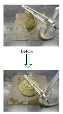
After Injection ratio : 17% Mini slump test : 7.5cm
