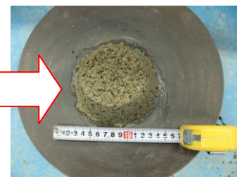
After adding TG Rock 1.5 kg/m 3 Table flow value 10.5 cm x 10.5 cm
