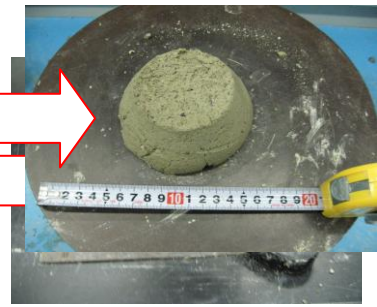
After adding TG Rock-L 1.0 kg/m 3
