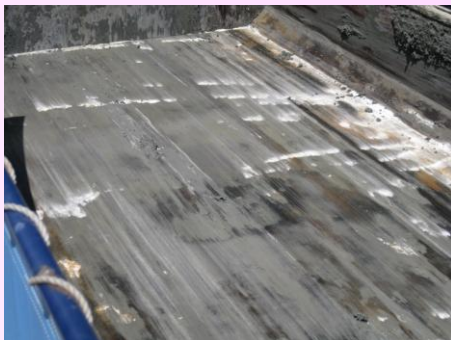
After unloading soil No adhesion of soil
