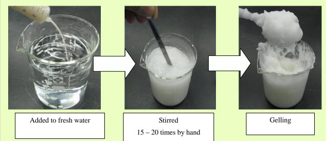
When TG Jeru is dissolved into water, due to the thickening and water retaining effects thereof, the water forms a gel as shown in the above photos. With such effects, TG Jeru exhibits the effects of blocking water in strata of high permeability and in the event of a blowout.
